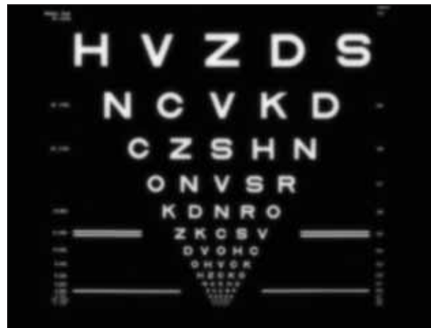
0.3µm spherical aberration on paraxial focus
